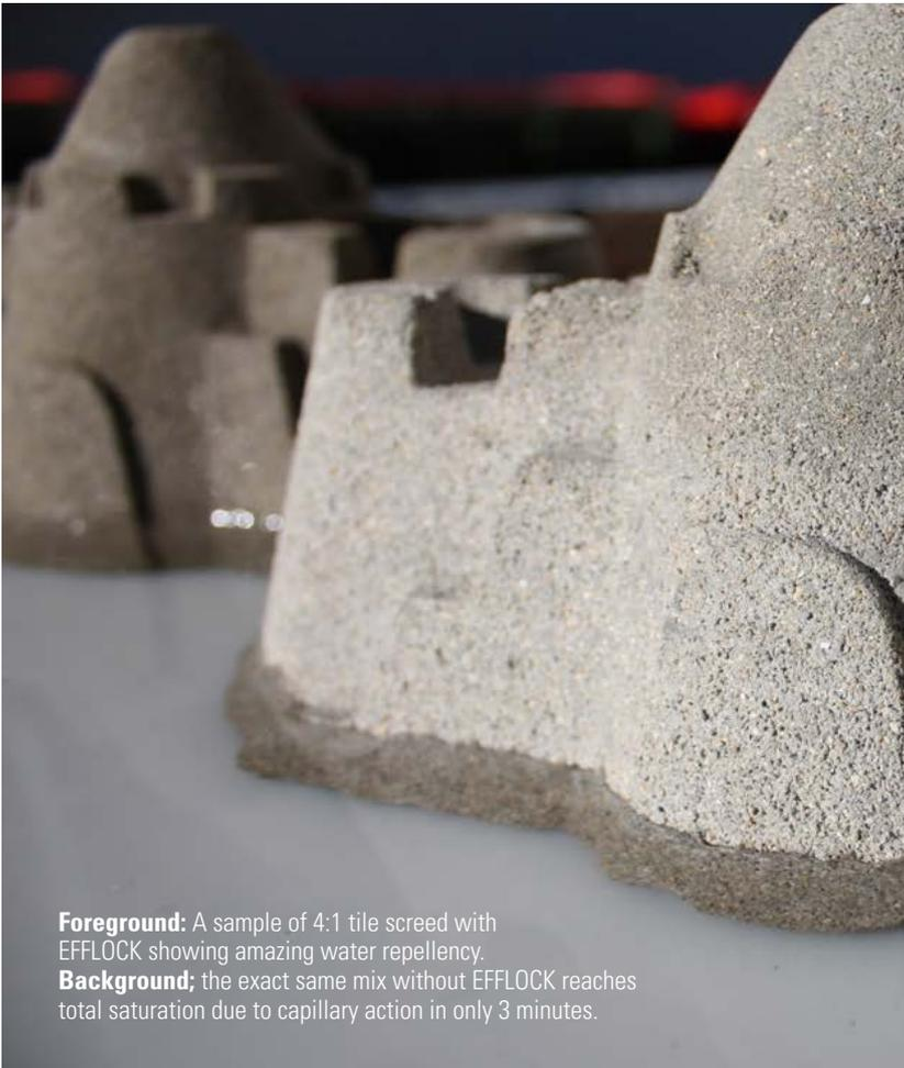
**Foreground:** A sample of 4:1 tile screed with EFFLOCK showing amazing water repellency.
